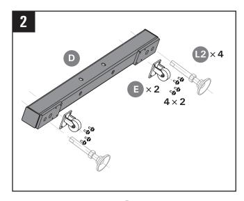
Assemble two casters **E** with 8 small fasteners sets onto the cross beam **D**. Screw in the two shorter levelers **L2**.
