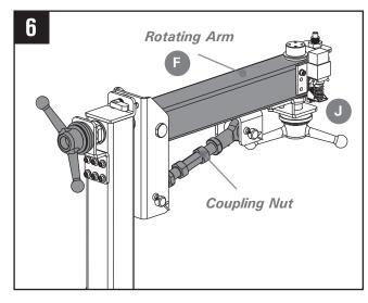
First level the frame base with the three levelers on the ground. Then level the Rotating Arm F by turning the coupling connector J.
