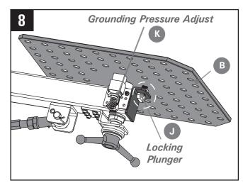
The turn table **B** should be locked with PLUNGER **J** engaged, after the top is installed. Adjust the GROUNDING CONTACT **K** pressure with spring position setting.
