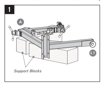
Place the main farm A on some support block or table edge. Make sure the parts are stable.
