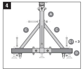
Connect the two side support C to the main frame Assembly A + D with three larger/longer fasteners.
