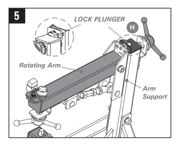
IMPORTANT: To prevent the table top flip, the rotating arm should be LOCKED with the PLUNGER H before installing the heavy top plate.
