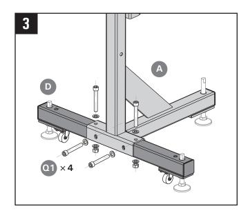
Assemble the Cross beam D to the main frame A with four larger/longer fastener set. Tighten the fasteners after they are fully aligned. A helper may be needed for safety.
